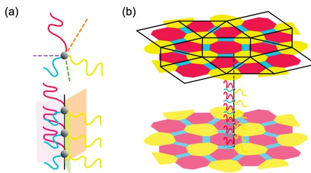
FIG. 1 (color). Schematic drawings of the intramolecular phase separation of *ABC* star-shaped terpolymer chains in bulk (a) and their nanodomain assembly (b). When the three phase-separated components are strongly incompatible with one another, the junction points are aligned on lines in bulk. Accordingly, the components tend to form microphase-separated structures with cylinder-based morphology.
