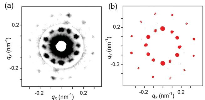
FIG. 4 (color). (a) The microbeam small-angle x-ray scattering pattern obtained for the annealed sample film of  $I_{1.0}S_{2.7}P_{2.5}$  with approximately  $30 \mu\text{m}$  thickness. The intensities of the outer 12 diffraction peaks are scaled up by a factor of 10. (b) The simulated diffraction pattern for Fig. 3(b) displaying only peaks above an arbitrary intensity. The radii of circles are proportional to their intensities.
