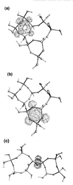
FIG. 3. Examples of the valence molecular orbitals localized in (a) four-, (b) three-, and (c) two-membered silica rings.
