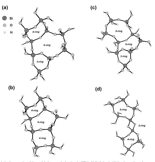
FIG. 2. Optimized geometries of the model clusters calculated at the HF/6-31G(d) level. All the clusters have the same stoichiometry of Si<sub>9</sub>O<sub>25</sub>H<sub>14</sub>: (a) Model 3-4-6, (b) model 4-4-5, (c) model 3-5-5, and (d) model 2-4-5.
