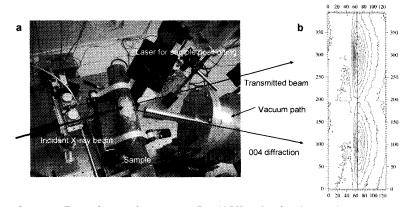
Fig 1 a: Experimental setup at BL40XU, SPring8, Harima, Japan. The log was tightly fixed being tilted ca.15° with respect to the incidence so that the (004) planes satisfy Bragg condition. The vacuum path of 1.5 m was inserted to suppress the background due to the air scattering.
