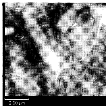
Fig. 1. AFM image of bacterial cellulose pellicle (bar: 2 \mu m)
