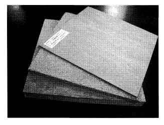
binderless boards was excellent while the board density were relatively low. The mechanical performance of binderless boards was improved with increasing the steam pressure and the longer pressing time contributed to the better dimensional stability. The chemical changes and self-bonding characterization of kenaf core is also investigated.
