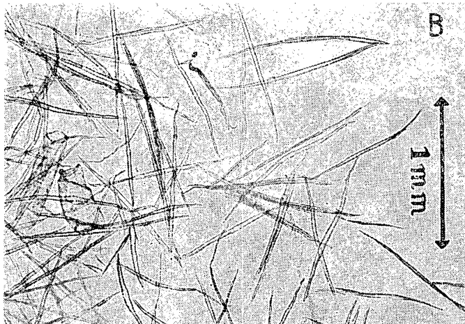
Phot.(B) Screened unbleached kraft pulp of "Akamegashiwa" ( Mallotus japonicus Muell. Arg.) Mean fiber length 0.915mm
