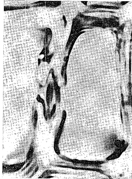
F. Unaspirated pit-pair. Latewood, \times , 1600 \times .
