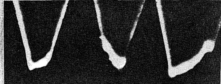
Photo. 2. Pictures of edges before and after cutting about 8 m of beech, Japanese cypress and red lauan (by means of optical slit method).
