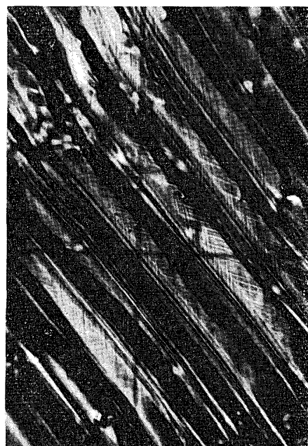
Photo 24. Spiral cracks of compression wood. They appear at ca. 45^\circ to tracheid axes, but no slip line can be found. AKAMATSU, ( r ), \times 310
