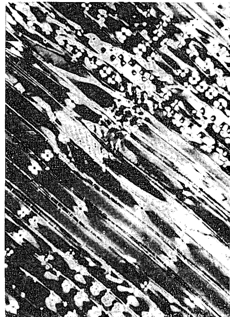
Photo 20. In outer surrounding part of a test piece of rotary bending, the compression and tensile stress are alternately repeated, and accordingly many slip lines take place and reach from radial to tangential cell wall and to adjacent cells continuously. HINOKI, ( r ), \times 160
