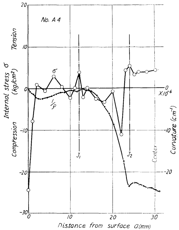
Fig. 3 (4). Plots of measured curvature and calculated stress in the glued laminated wood (No. A 4).
