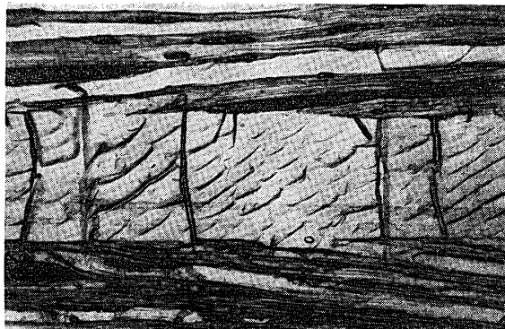
A. Glue-line thickness : ca. 250\mu , t
