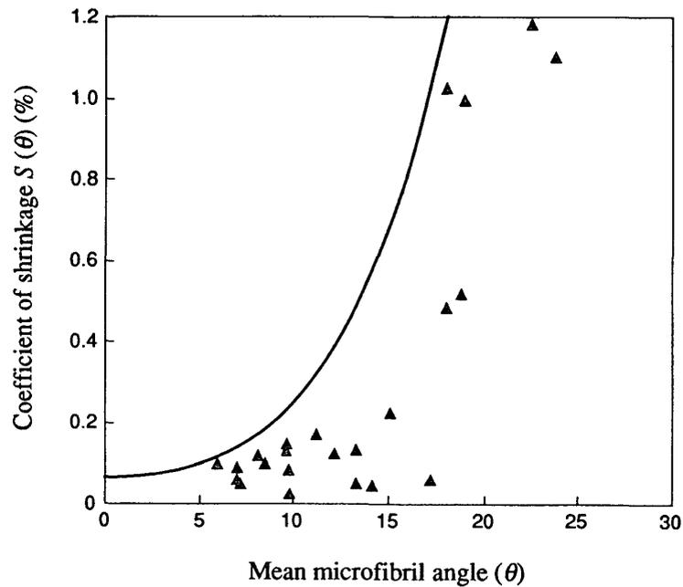
Fig. 2. Comparison between the calculated (solid line) and experimental (▲) values of  $S(\theta)$ .
