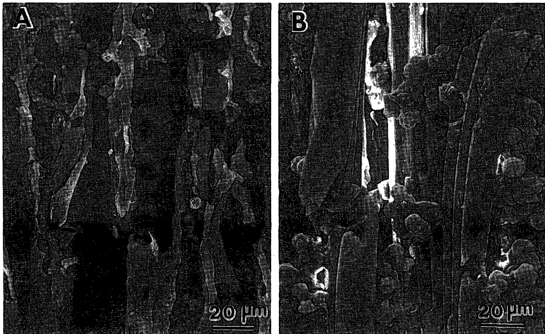
Fig. 7. Surfaces of untreated (A) and acetylated wood (B) after one year of weathering tests under outdoor conditions.
