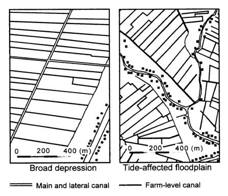
Fig. 4 Farm-level Canal Layout
