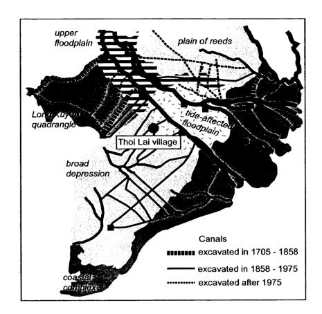
Fig. 1 Canal Layout in the Mekong Delta
