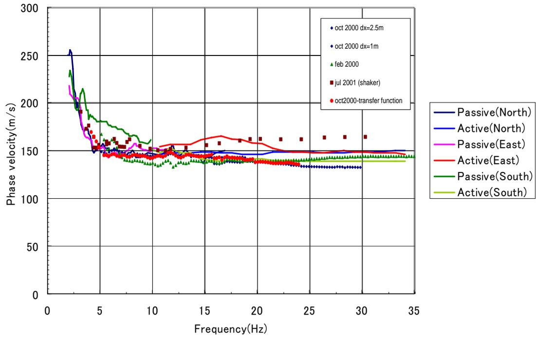
Figure 5.4.7 Comparison of dispersion curves with Foti (2003).
