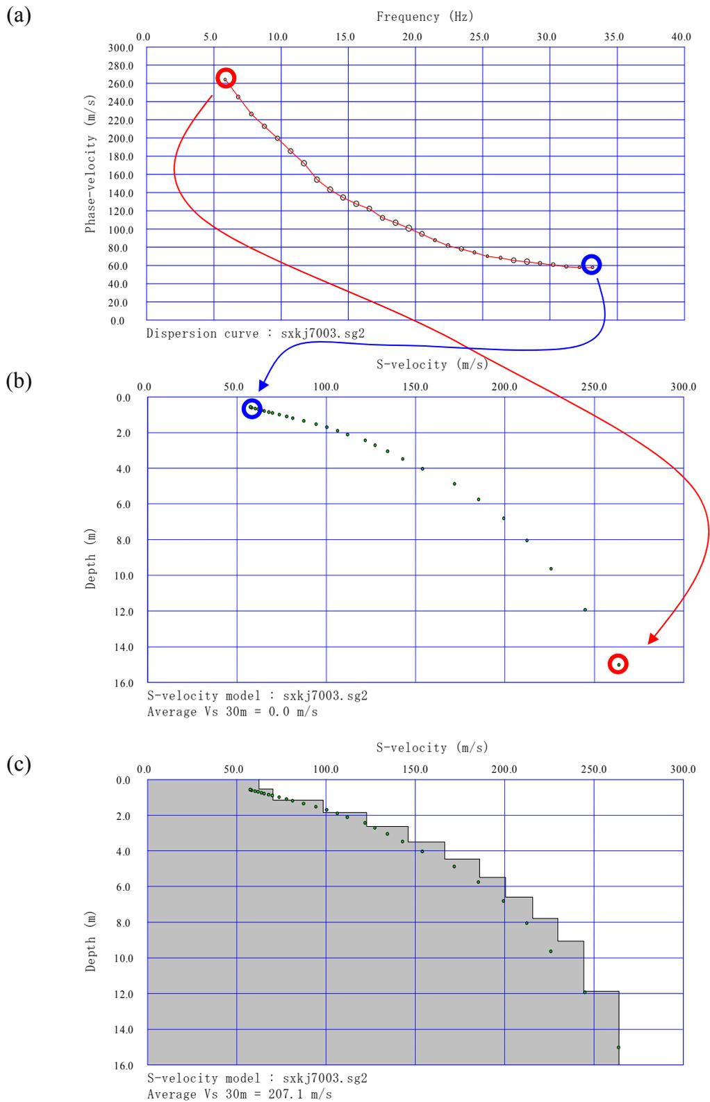
Figure 2.8.3 Initial model based on 1/3 wavelength transformation.
