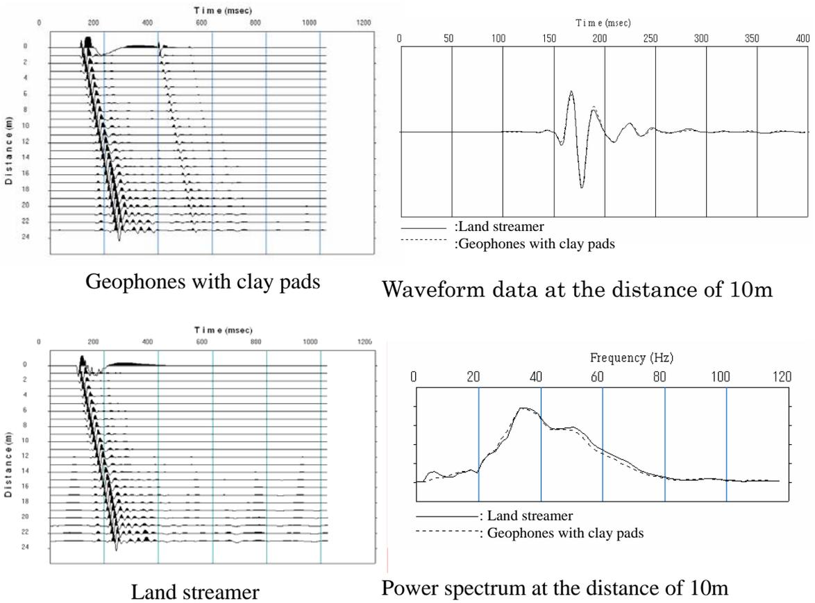
Figure 5.6.2 Comparison of common shot gathers obtained on a paved road at the top of a levee.
