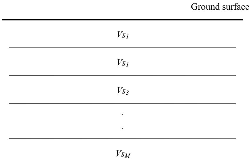
Figure 2.8.1 A one-dimensional  $M$  layers S-wave velocity model.
