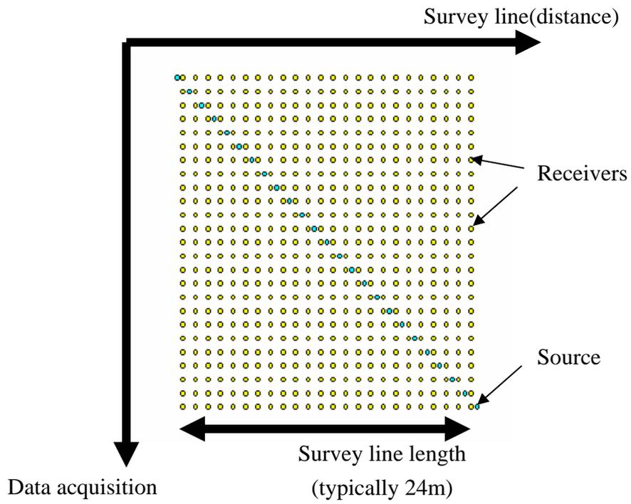
Figure 5.2.1. Typical source-receiver geometry used in housing site investigations.
