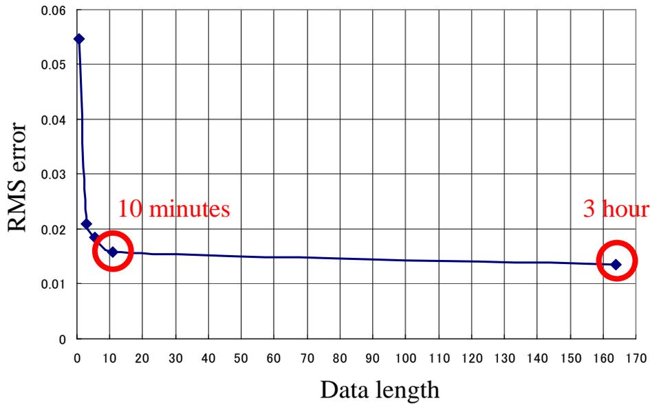
Figure 4.2.5 Root mean square error against data length.
