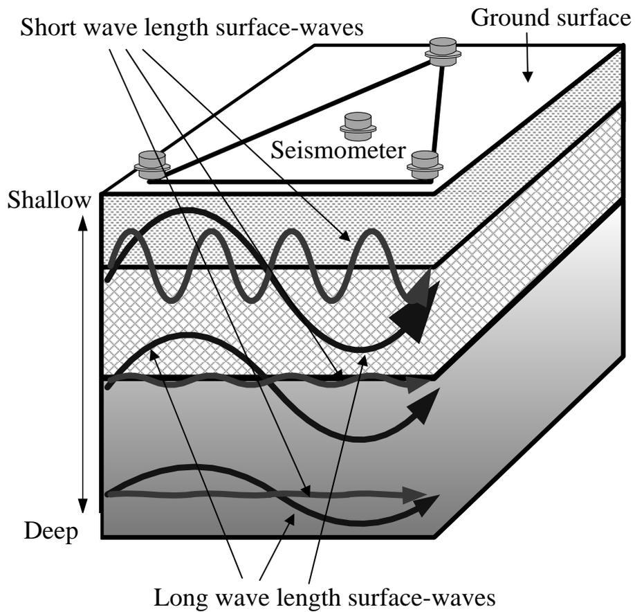
Figure 4.1.1. Schematic diagram showing microtremor array measurements. Amplitude of shorter wave length surface-waves decay rapidly with depth whereas one of longer wave length keep amplitude even if deeper part. Therefore, shorter wave-length surface-waves reflect shallow S-wave velocity and longer one reflect deeper S-wave velocity. S-wave velocity profile can be estimated by measuring phase-velocity for different wave-length (frequency).
