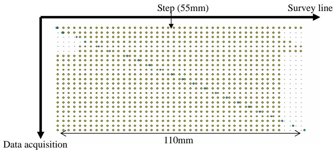
Figure 3.4.15. Source and receiver geometry for CMPCC analysis. Blue circles indicate sources and yellow circles indicate receivers.
