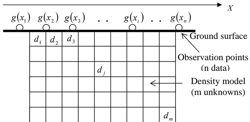
Figure 5.3.2. Two-dimensional density model used in an analysis.
