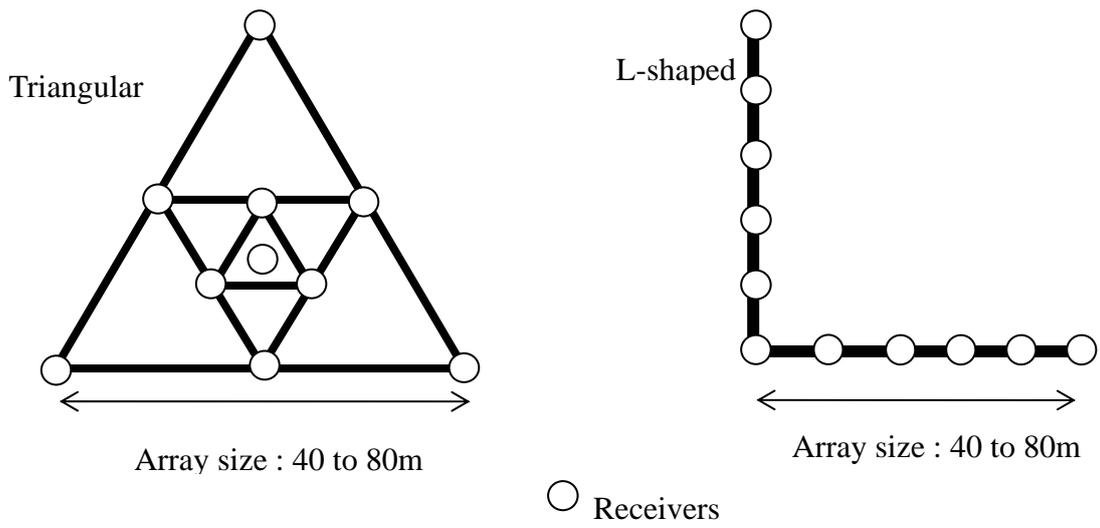
Figure 5.8.3. Receiver arrays used in the passive method.
