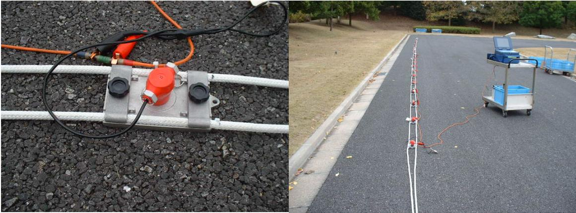
Figure 5.6.1 Land streamer for a surface-wave method.
