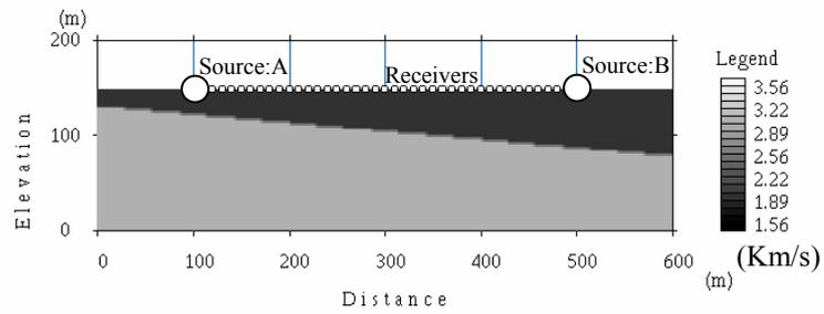
Fig.2.5.1. The slope model used in the numerical simulation. The figure shows the P-wave velocity model.
