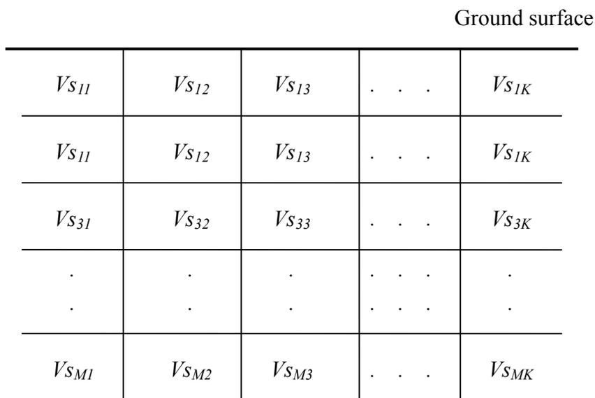
Figure 2.8.2 A two-dimensional  $M$  layers S-wave velocity model.
