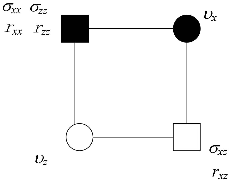
Figure 2.4.2. The two dimensional staggered finite-difference grid.  $\sigma_{xx}$  and  $\sigma_{zz}$  are normal stresses,  $u_x$  and  $u_z$  are particle velocities.  $r_{xx}$ ,  $r_{zz}$  and  $r_{xz}$  are memory variables.
