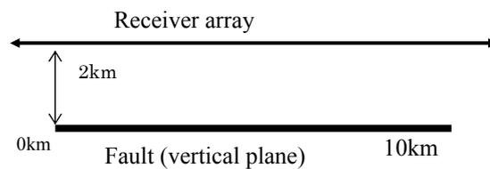
Figure 2.4.10. Finite-difference model used in the comparison of nonuniform-grid computation with uniform one.  $\Delta_z$  indicates grid spacing in  $z$  direction.  $Dx$  and  $dz$  indicate source spacing in  $x$  and  $z$  directions respectively. In the uniform-grid spacing,  $\Delta_z$  was set to 100m and  $dx$  and  $dz$  were set to 200m.
