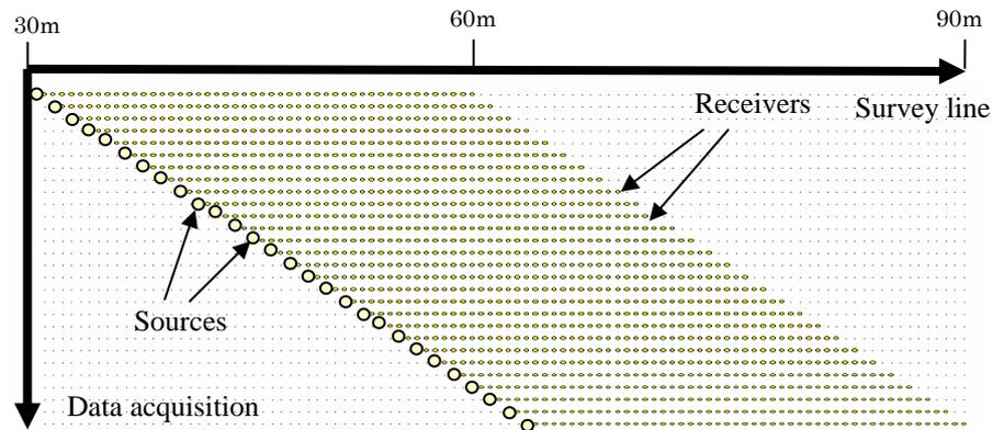
Figure 3.3.2. Source-receiver geometry used in a numerical test.
