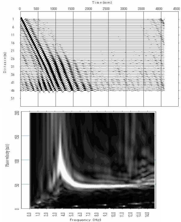
Figure 3.5.2. Result of CMPCC analysis for waveform data shown in the Figure 3.2.1. CMPCC gathers (top) and their phase-velocity frequency images (bottom). CMP distances are 173m (a) and 201m (b).
