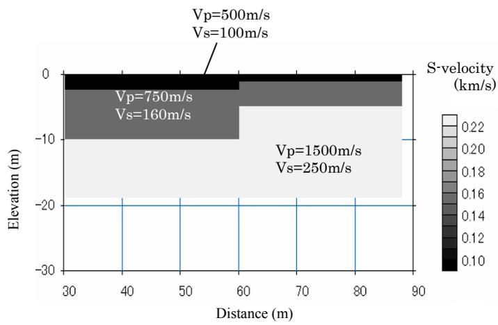
Fig.2.5.10. The step model used in the numerical simulation. The figure shows the S-wave velocity model.
