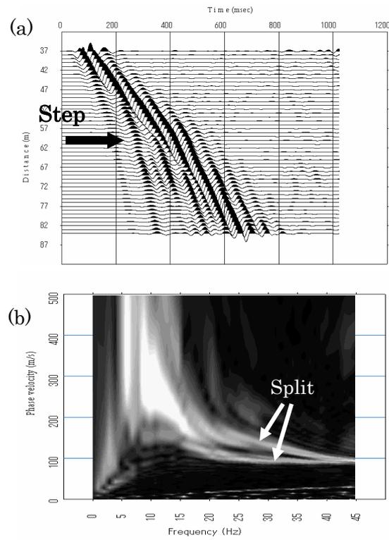
Figure 3.3.3 Shot gathers (a) of 35.8m shot and its phase-velocity frequency image (b).
