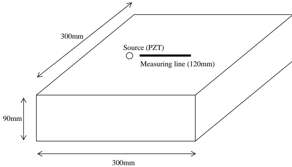
Figure 3.4.2. Source-receiver configuration used in the experiment. A source and a measuring line are placed in the middle of the models. Waveforms are collected at the surface of the models with 4m distance interval.
