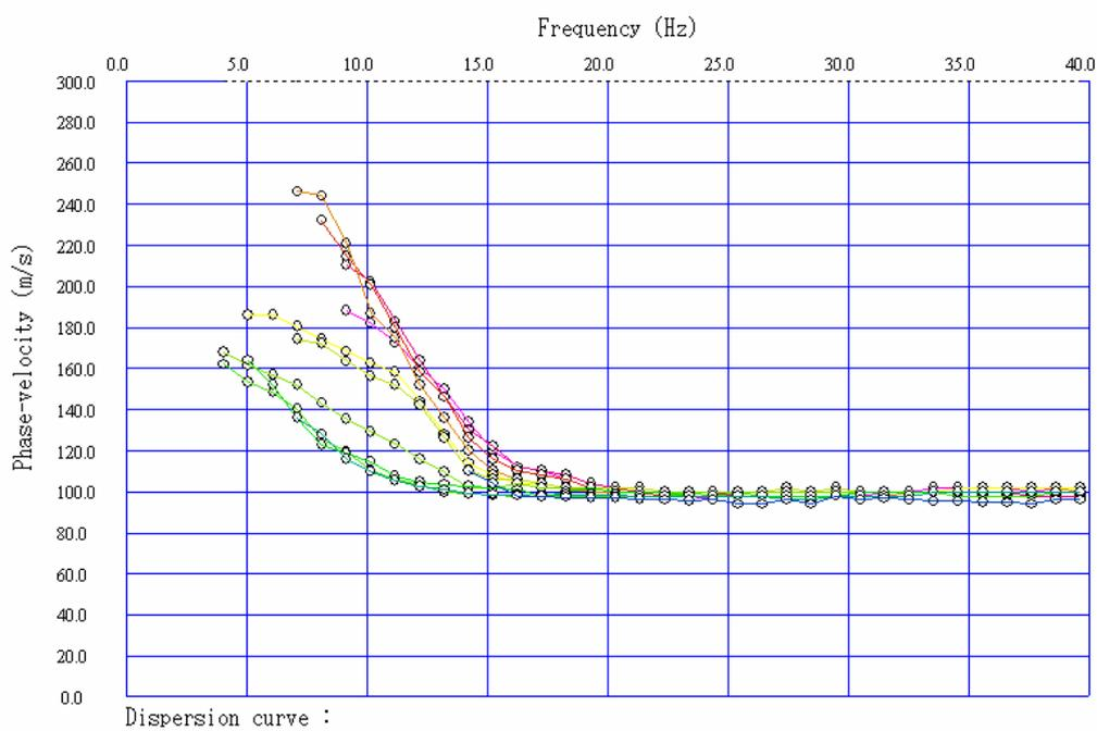
Figure 5.2.6. All dispersion curves for CMPPC gathers. Red to yellow dispersion curves indicates first half and green to blue curves indicates latter half.
