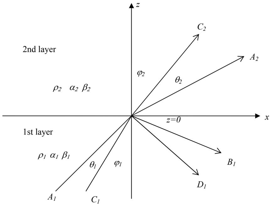
Figure 2.3.5 Boundary condition of P-SV wave between two layers.
