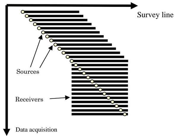
Figure 3.2.4. A source-receiver geometry of moving-source observation for CMP analysis of surface-waves.
