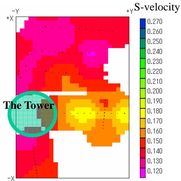
Figure 5.4.23. Plan views of interpolated S-wave velocity model around the Tower.
