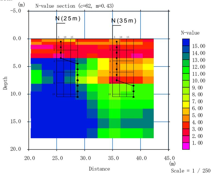
Figure 5.2.9. Converted N-value profile using estimated  $m$  and  $c$  ( $m=0.43$ ,  $c=62m/s$ ).
