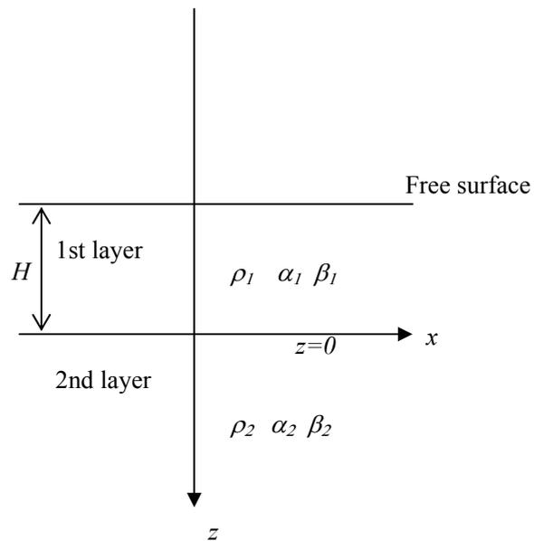
Figure 2.3.6 Two layer model for Rayleigh waves.  $\rho$ ,  $\alpha$  and  $\beta$  are density, P-wave velocity and S-wave velocity respectively..
