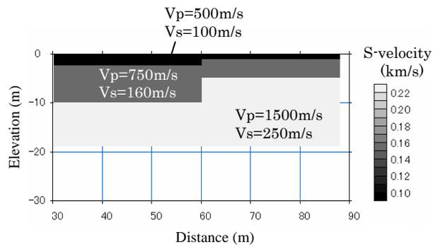
Figure 3.3.1. Velocity model used in a numerical test.
