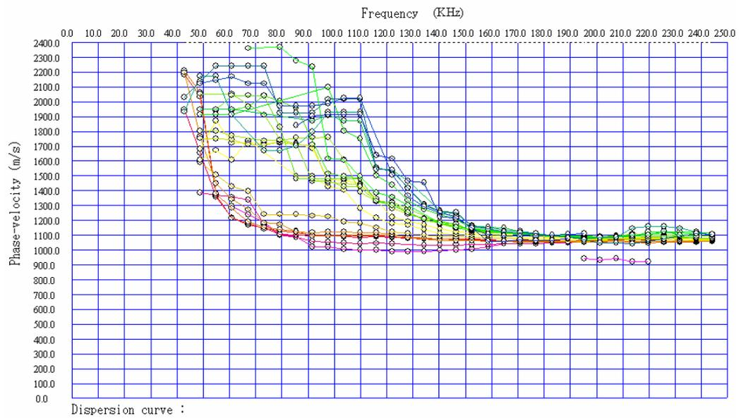
Figure 3.4.18. All dispersion curves calculated from CMPCC gathers. Difference of color indicates the difference of CMPCC location. Red to yellow curves are placed in left side of the step and green to blue curves are placed in right side of the step.
