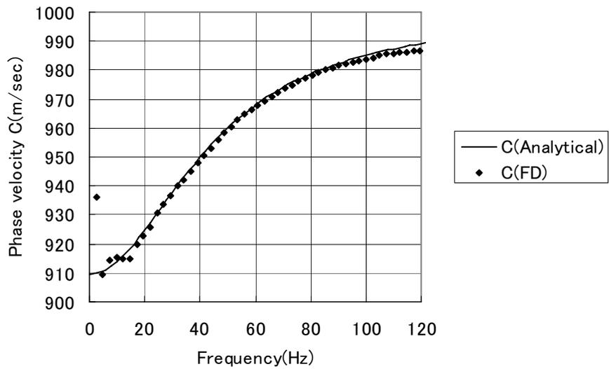
Figure 2.4.6. Comparison of quality factor  $Q(\omega)$  and phase velocity  $C(\omega)$  obtained from finite-difference method with analytical solutions. Dots indicate finite-difference solutions and solid lines indicate analytical solutions.
