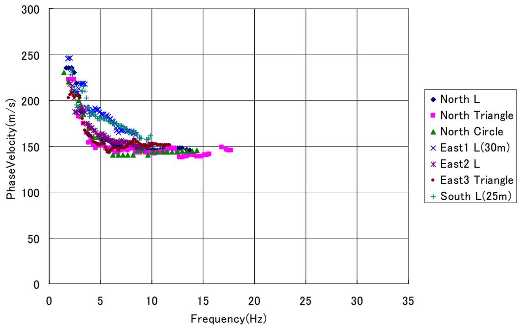
Figure 5.4.5 All dispersion curves obtained through passive method.
