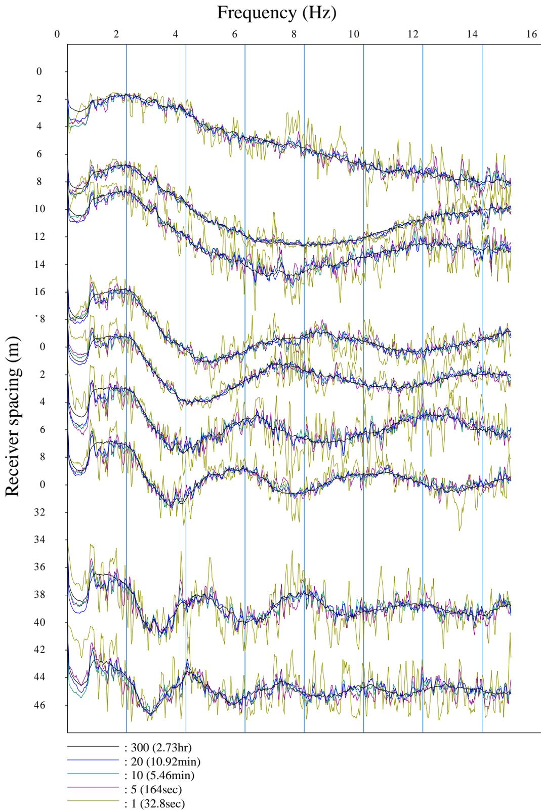
Figure 4.2.3 Coherence obtained from different record length data.
