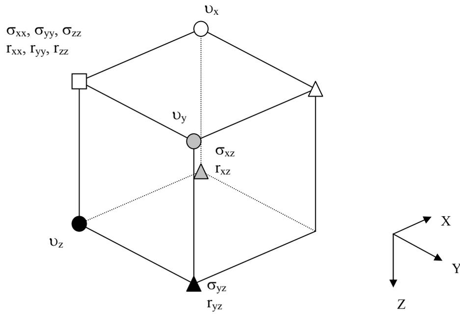
Figure 2.4.5. 3D velocity-stress staggered grid.  $\sigma_{ij}$  is  $ij$ <sup>th</sup> component of stress tensor,  $v_i$  is  $i$ <sup>th</sup> component of particle velocities,  $r_{ii}$  is  $ij$ <sup>th</sup> component of memory variables.
