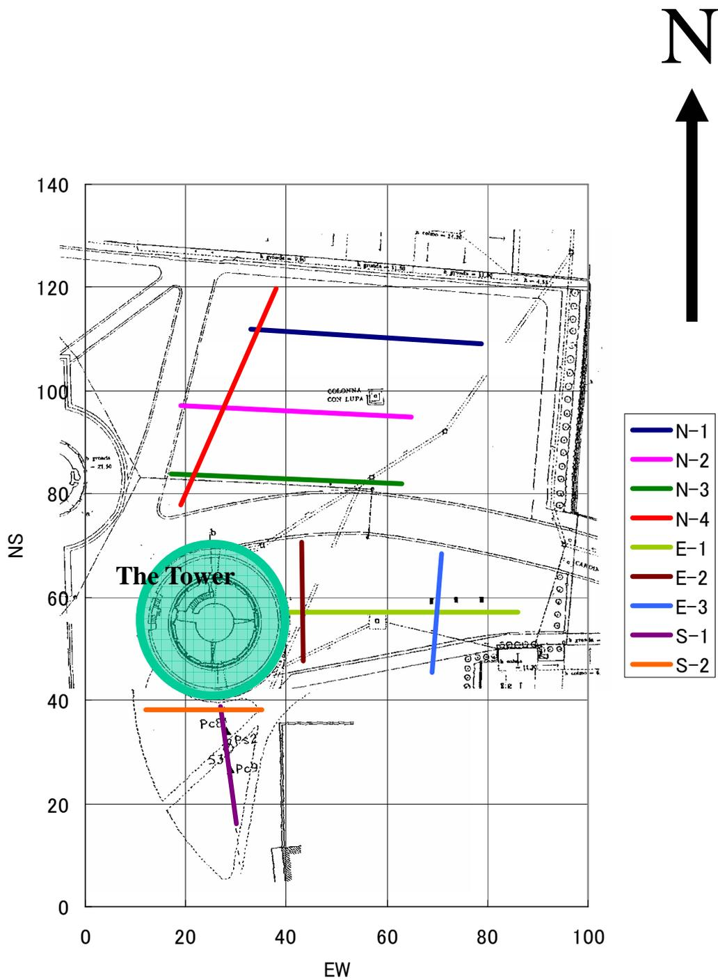
Figure 5.4.4 Location of active method survey lines.
