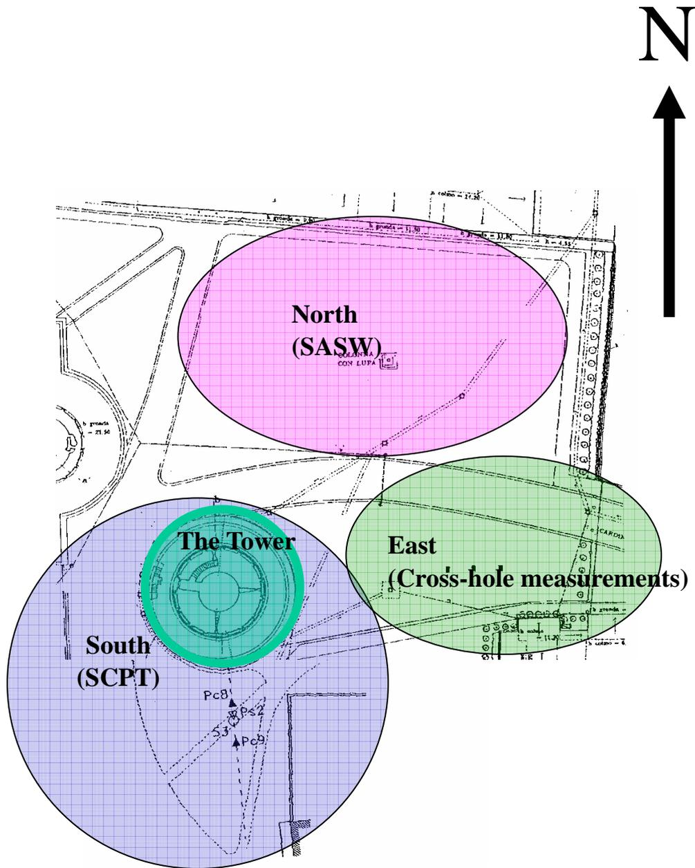
Figure 5.4.2 Description of the site and S-wave velocity measurements already performed at the site.
