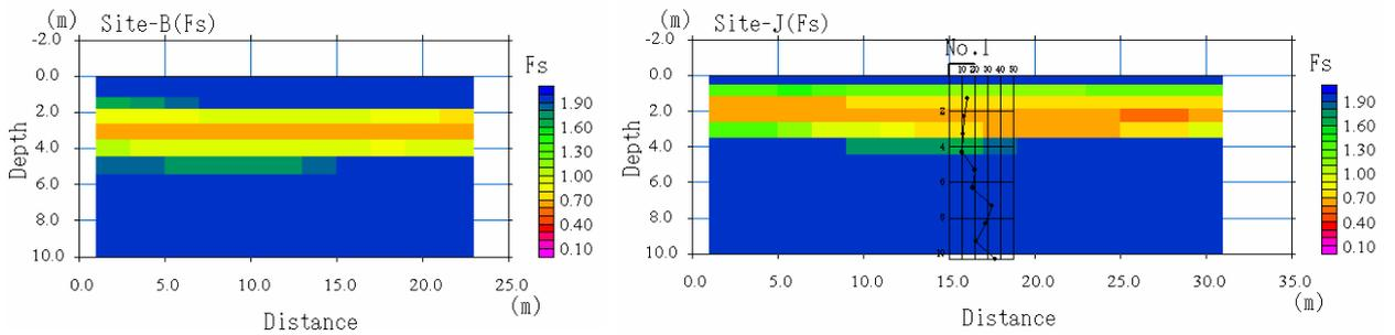
Figure 5.5.8. Factor of safety (Fs) models calculated from the CRR and the CSR for the site B (left) and J (right).
