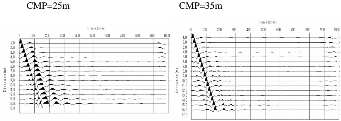
Figure 5.2.4. CMPCC gathers for the CMP distance of 25m(left) and 35m(right).
