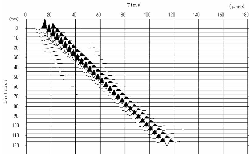
Figure 3.4.6. Synthetic waveform calculated by 3D elastic finite-different method.  $V_p=2500\text{m/s}$ ,  $V_s=1300\text{m/s}$ , density= $1500\text{kg/m}^3$ , grid spacing= $0.5\text{m}$ . P-wave source with  $100\text{KHz}$  Ricker-wavelet is used.
