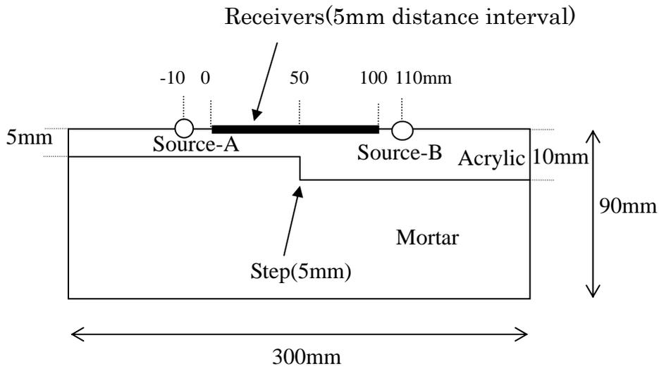
Figure 3.4.11. A two-dimensional model used in the experiment.
