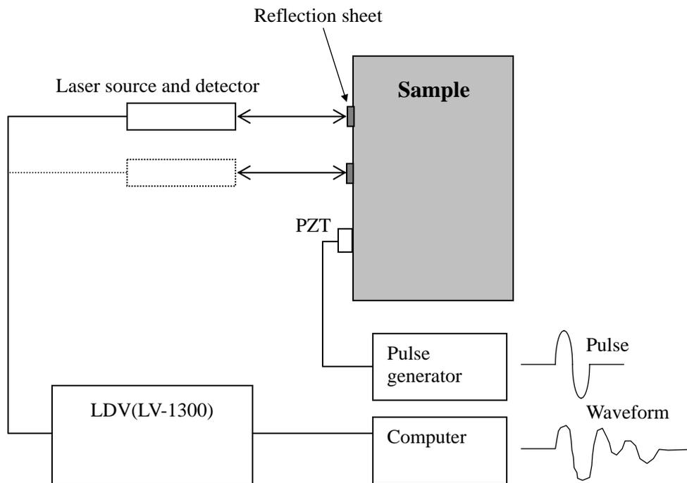
Figure 3.4.1. Schematic diagram of the measurement system using a laser Doppler vibrometer (LDV) and a piezoelectric transducer (PZT). The PZT is mounted on the surface for generating elastic waves. The laser beam illuminates the high-gain reflection sheet, which reflects the beam in an incident direction.
