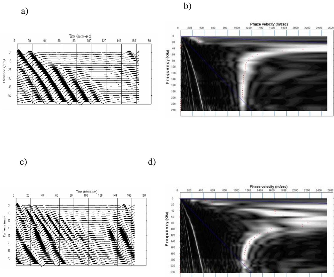
Figure 3.4.17 Example of CMPCC gathers. (a) Waveforms and (b) phase-velocity frequency image for the CMP distance of 27.5m. (c) Waveforms and (d) phase-velocity frequency image for the CMP distance of 72.5m.
