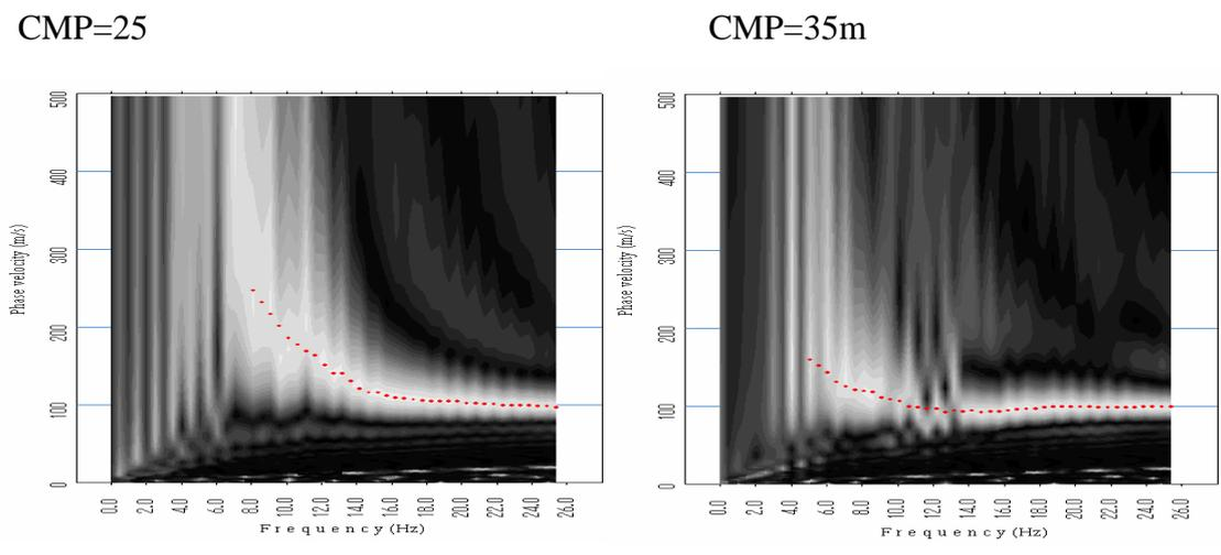
Figure 5.2.5. Phase-velocity frequency images of CMPCC gathers for the CMP distance of 25m(left) and 35m(right).
