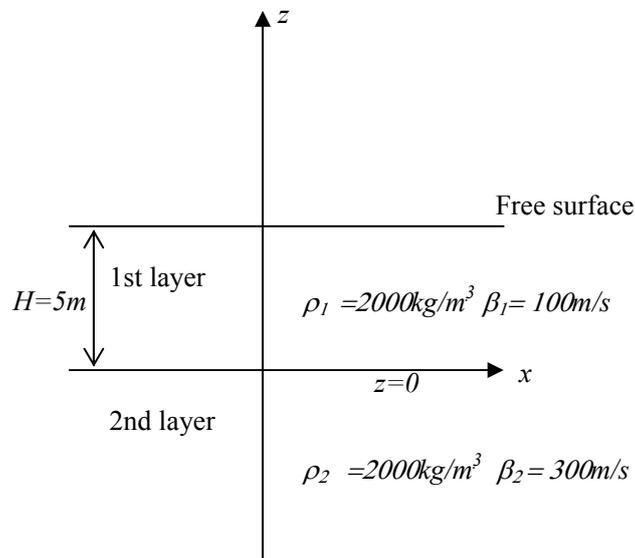
Figure 2.3.2 Example of two layer model for Love waves.  $\rho$  and  $\beta$  are density and S-wave velocity respectively.
