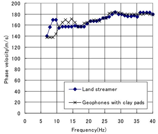
Figure 5.6.3 Comparison of phase-velocity image (left) and dispersion curves (right).
