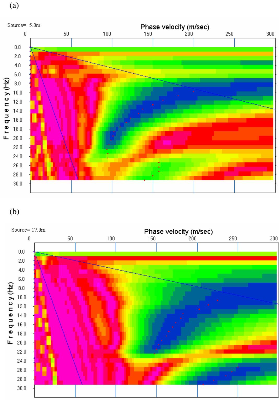
Figure 5.2.12 Example of phase-velocity images in frequency domain.
