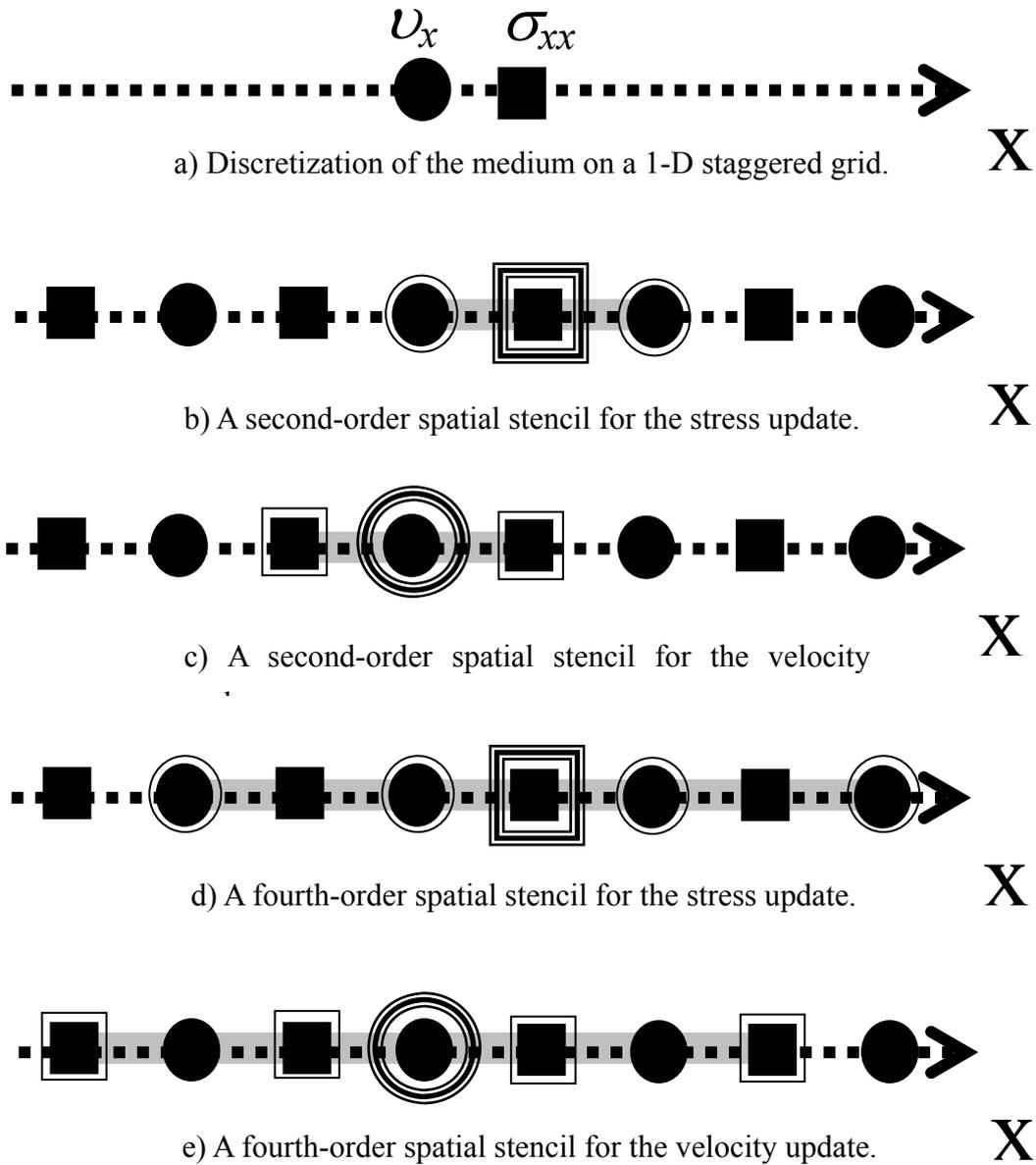
Figure 2.4.1. The one dimensional staggered finite-difference grid.  $\sigma_{xx}$  is a normal stress, and  $u_x$  is a velocity in x-direction.
