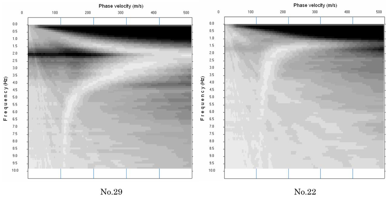
Figure 5.8.4. Example of phase velocity versus frequency.
