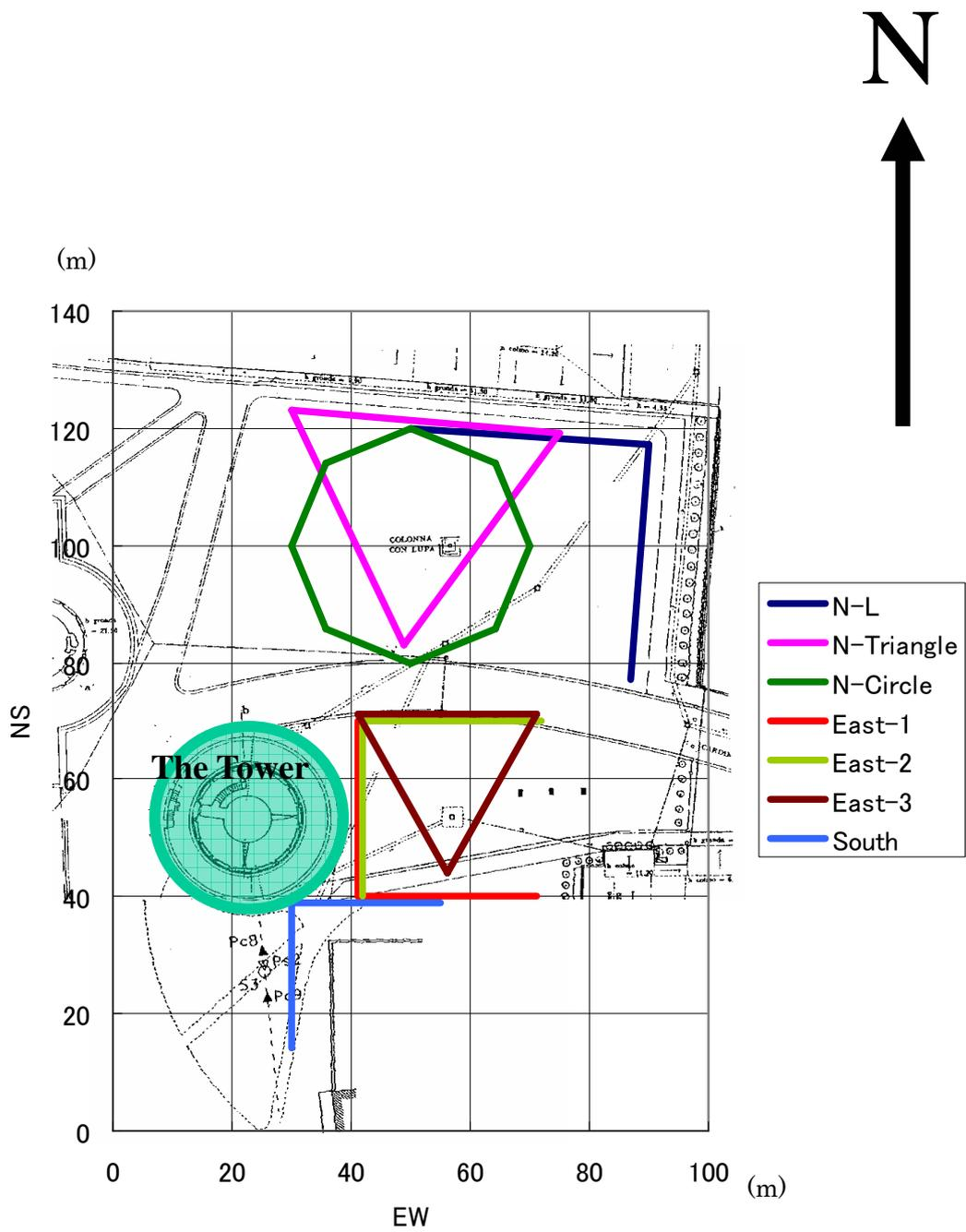
Figure 5.4.3 Location and shape of passive arrays.
