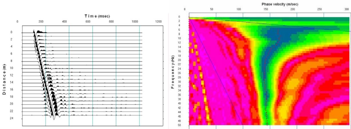
Figure 5.6.4 Example of waveform data (left) and its phase-velocity image in frequency domain (right).
