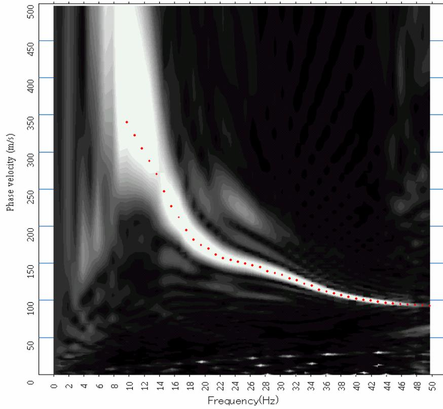
Fig.2.5.12. Image of dispersion curve (shot point 65.8m).
