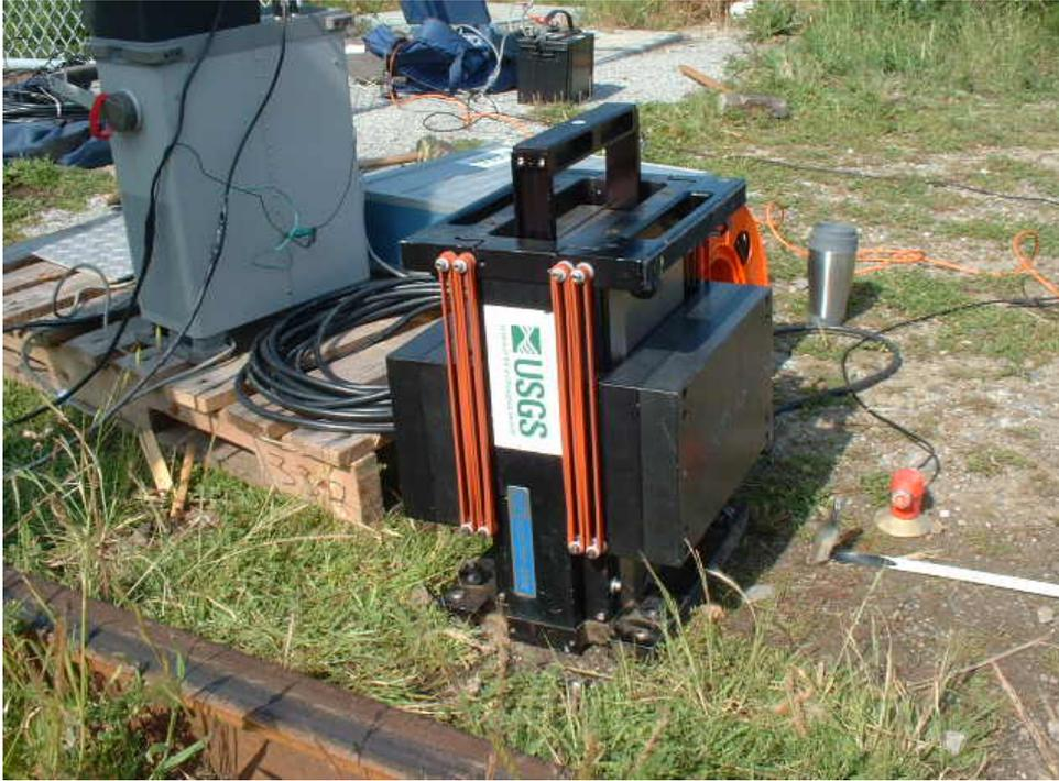
Figure 4.3.5 A typical shaker used in conventional surface-wave
