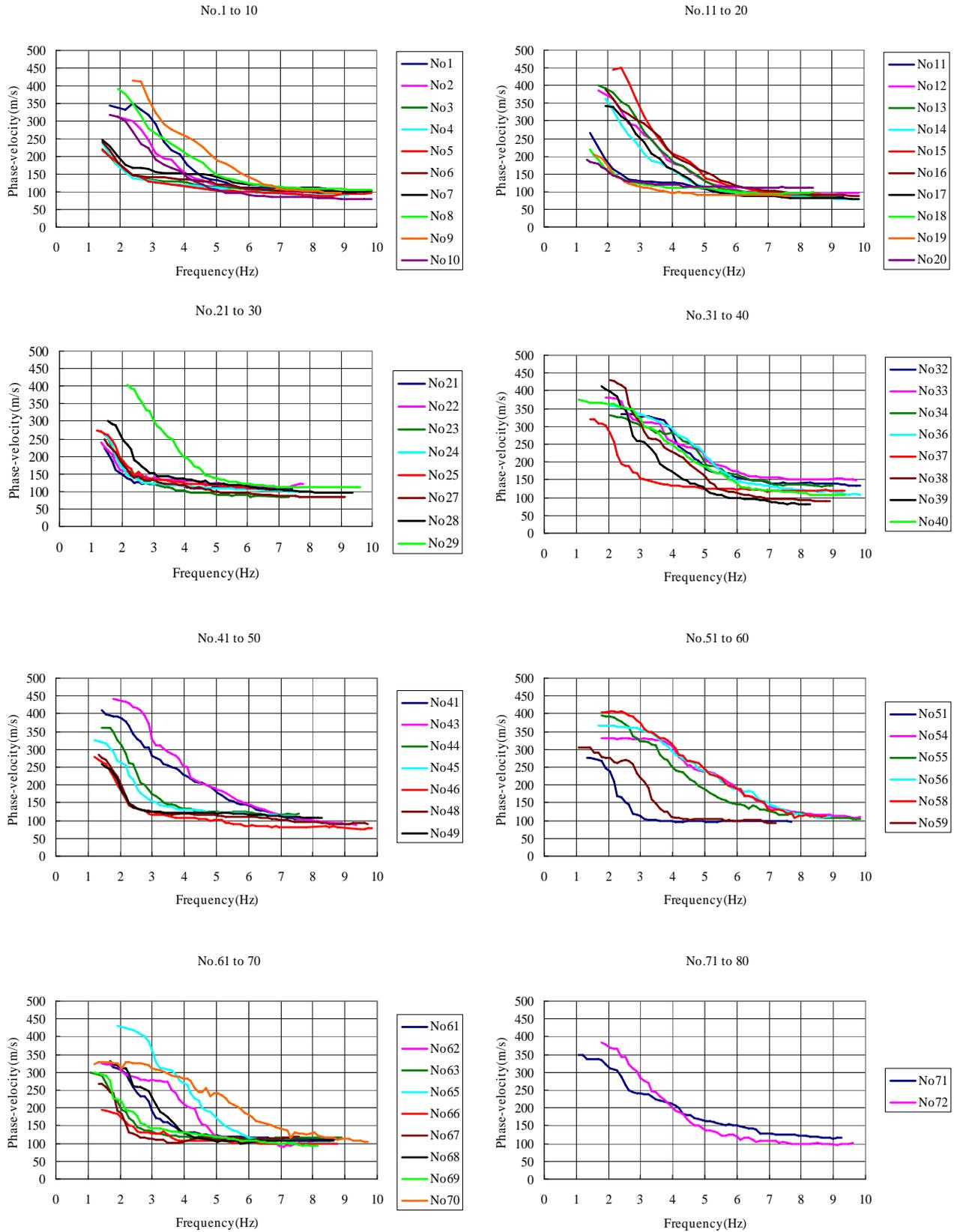
Figure 5.8.6 Dispersion curves for all 104 measurements points.
