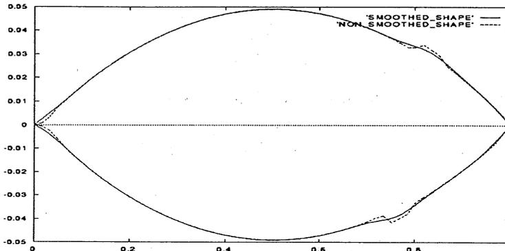
Figure 1: *Smoothed and unsmoothed shapes. We can see that the gradient jumps through shocks and also produces a non-smooth shape in leading edge regions. This is the result of the first iteration of the optimization. If we keep continue the shape becomes more and more irregular.*
