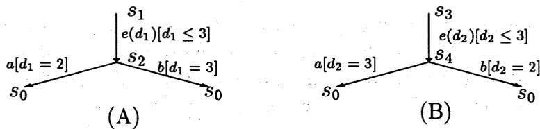
Figure 4: Example of A-TSLTS where  $s_1$  and  $s_3$  are not untimed bisimulation equivalent.
