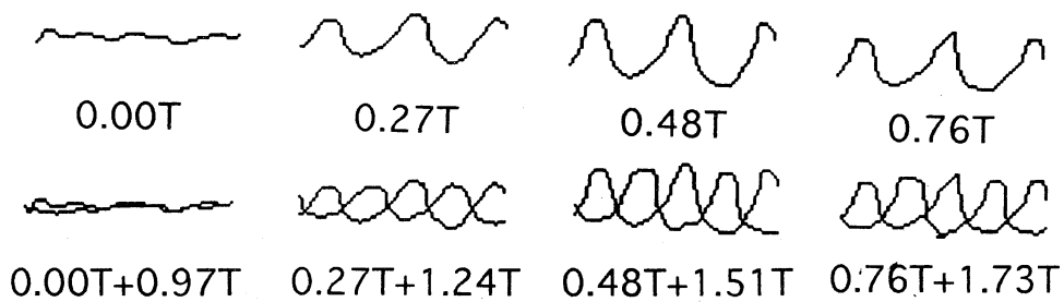
図9. 自由表面の輪郭; \eta \approx 8, \Gamma = 5.4 (f = 35\text{Hz}, a = 1.1\text{mm})
