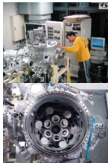
Multi-cathode helicon sputtering apparatus and the preparation chamber (top view).
