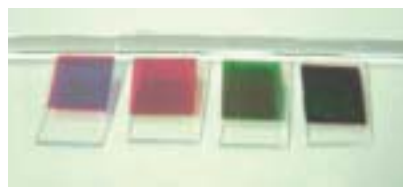
The dual-periodic multilayer structures with various thickness-modulation parameters. These layers are clearly uniform and the colours are somewhat beautiful.
