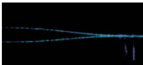
Y-branch channel waveguide directly written by UV laser irradiation. Ar + laser light (488nm) is coupled.
