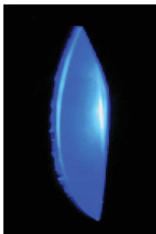
Figure 1. Cathode luminescence of SrTiO 3 .
