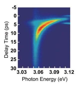
**Figure 2.** Time-resolved PL spectra of the In<sub>x</sub>Ga<sub>1-x</sub>N thin film.
