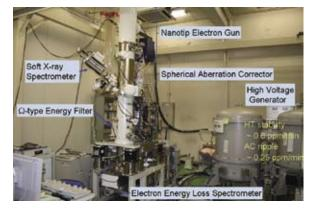
Figure 1. A 200kV TEM/STEM with nanotip electron gun.
