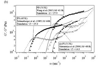
Figure 2. (a) A typical snapshot of the simulation and (b) the prediction of linear viscoelasticity for various polymer melts.
