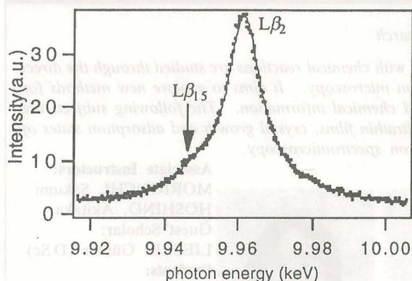
**Figure 2.** Spectrum of  $L\beta_2$  and  $L\beta_{15}$  line. Tube voltage is 30 kV, tube current is 15 mA. Crystal is Si(333) and  $2\theta$  is 73.13 degrees. Dots are measured value and solid line is fitted by lorentzians.
