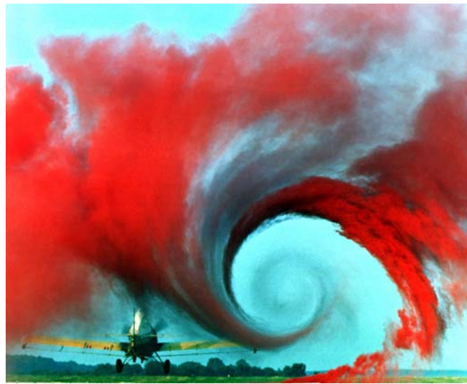
Fig. 6.4 A smoke picture of wing-tip vortex observed in the wake of an agricultural aircraft
