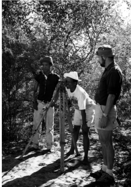
Fig. 4. The writer gives a lesson in use of the dumpy level to /Ui and Royal, Cho/ana.
