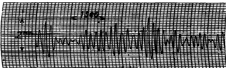
Fig. 6 A record of wind waves measured by wave meter for small amplitude
