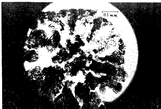
Photo. 1. Slice of prilled AN by optical microscope.
