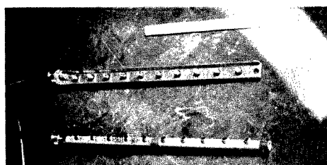
Photo. 1 Array of photo-cell elements and lamps of D-1 type sediment meter.
