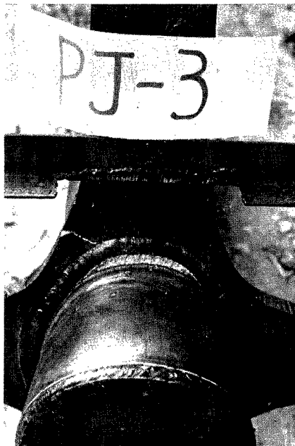
Photo. 7 Failure of stiffener in "tension type" specimen PJ-3.
