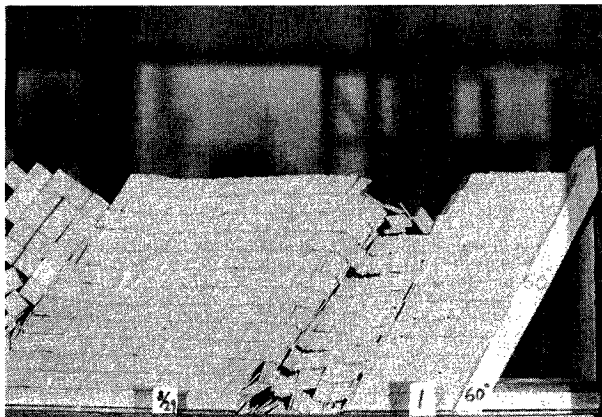
Photo. 12 Pattern of failure with buckling in steeply inclined strata. \theta = 60^\circ .
