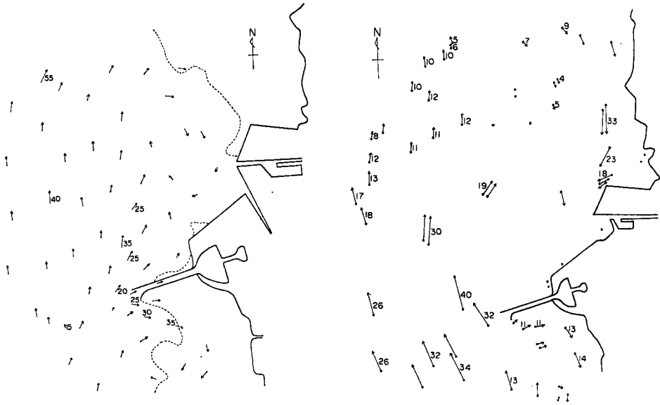
Fig. 2 (a) Flow pattern at high water in the Omuta area, numeral means velocity in cm/sec (prototype).
