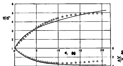
Fig. 32 Relationship among \sigma_1/\sigma_3, \epsilon_1 and \Delta V/V in triaxial compression test on Ishii River sand.
