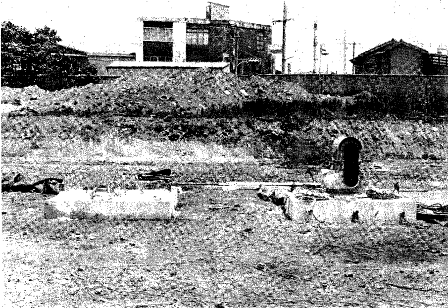
Photo. 2 Active (F2) and passive (F3) foundations
