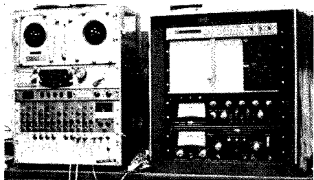
photo.2 Data-recorder and spectral analyzer
