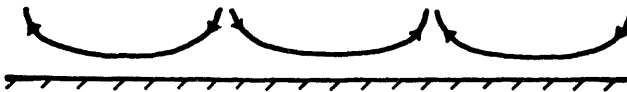
Fig. 4. Correlation of inflow with lateral stretching, and outflow with lateral compression, of vortex lines after Lighthill.
