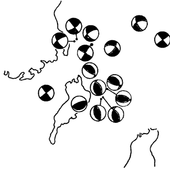
Fig. 6. Distribution of earthquakes mechanism in the northern area around Lake Biwa, open parts; dilatation, solid parts; compression.
