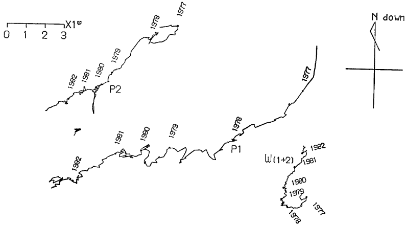
Fig. 5 Vector diagrams of secular variations of ground tilts observed at the Miyazaki Observatory. W_{(1+2)} is drawn from W-1 and W-2 data.
