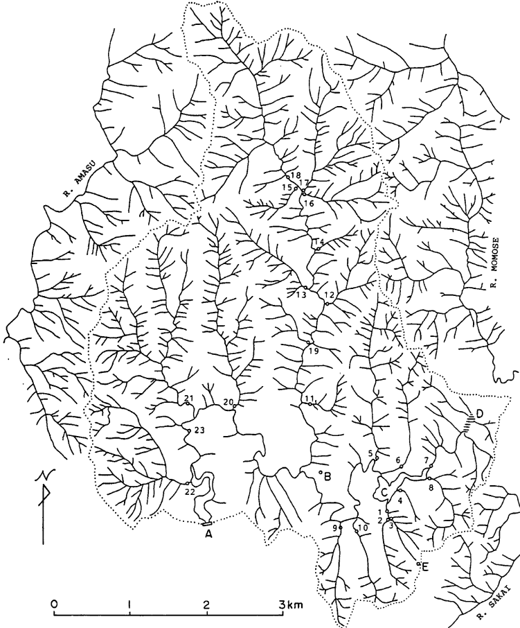
Fig. 1 Drainage network in the catchment of the Ishidagawa dam and its environs. A: Ishidagawa dam, B: Kochidani raingauge station, C: Tankai-ike reservoir, D: Hiraike swamp, E: meteorological station for snow observation. Circles with numbers indicate the stations for discharge measurement.
