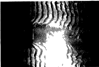
Photo. 5 Flow pattern around cylinder ( B/D=0.5 , Re=8.0 \times 10^3 , k=4 S_t ).
