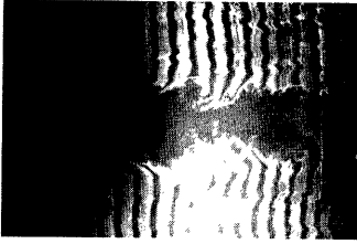
Photo. 17 Flow pattern around cylinder ( B/D = 2, Re = 8.2 \times 10^4, k = 4S_t ).
