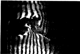
Photo. 11 Flow pattern around cylinder ( B/D = 1 , Re = 7.3 \times 10^3 , k = 0 ).
