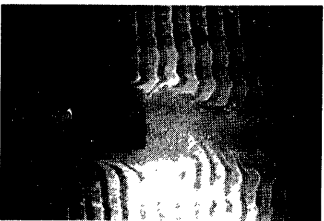
Photo. 15 Flow pattern around cylinder ( B/D = 2 , Re = 8.3 \times 10^3 , k = 0 ).
