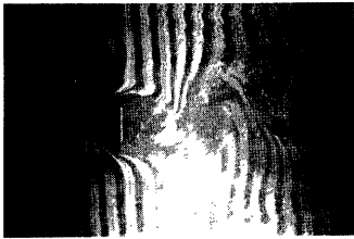
Photo. 1 Flow pattern around cylinder ( B/D=0.5 , Re=8.3 \times 10^3 , k=0 ).
