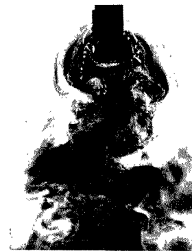
Photo. 5. End view of vortex formation at Reynolds number 1 \times 10^3 and aspect ratio 2.0.
