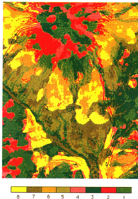
Fig. 11 Landform classification of the southern part of the Yatsugatake Volcano area using DEM.
