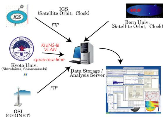
Fig.6. The flow of information of the semi-real time monitoring system.
