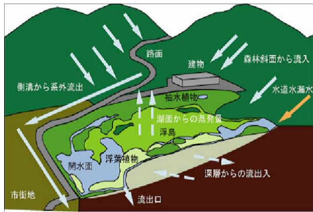
Fig. 4 Conceptual image of water balance of the pond
