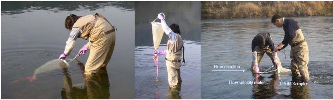
Photo 3 Scene of SPOM sampling using POM net in running waters taken in Uji River
