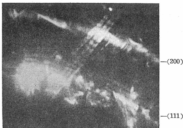
Fig. 1. Diffracted spots accompanied by subsidiary spots of intensity maxima found in the Debye-Scherrer rings of (111) and (200) planes obtained from the "Trigon" particles (camera length : 800 cm).
