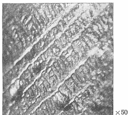
Fig. 5. Microstructure of side surface, (001). showing the cross partial dendrite structure. Lowering speed, 14 mm/min.
