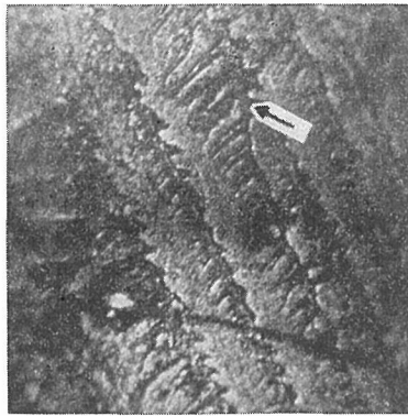
Fig. 13. Microstructure of side surface of the specimen which was grown in the direction inclined at 20^\circ from [110] to [100] . Lowering speed, 14 mm/min.
