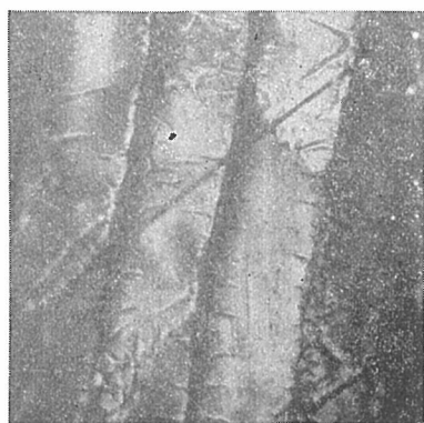
Fig. 11. Microstructure of side surface of the specimen, (001), which was grown in the direction inclined at 10° from [110] to [100]. Lowering speed, 0.7 mm/min.
