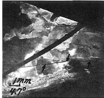
Fig. 14. X-ray micrograph of the side surface (100) of the specimen (99.98% pure tin) in parallel to [001] at 0.13 mm/min and 45°/cm. Fe K\alpha , reflecting plane : (301).
