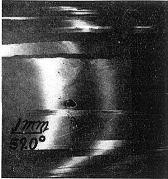
Fig. 13. X-ray micrograph of the side surface (001) of the specimen (99.98% pure tin) grown in parallel to [100] at 0.9 mm/min and 45°/cm. Fe K\alpha , reflecting plane : (103).
