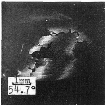
Fig. 15. X-ray micrograph of the cross section (001) of the specimen (99.98 % pure tin) grown in parallel to [001] at 2.5 min and 45°/cm. Fe K \alpha , reflecting plane : (103).
