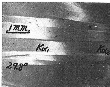
Fig. 8. X-ray micrograph of the specimen (99.87% pure tin) grown at 4 mm/min and 45^\circ/\text{cm} . Cu K\alpha , specimen face : (110), reflecting plane : (620).
